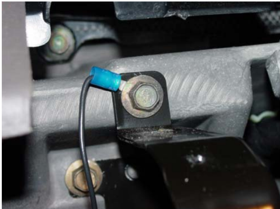
Figure 5. Make sure the ground is also connected to the vehicle.
